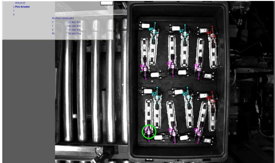
The Cognex suite of products also includes Cognex Connect software and as a complete solution, enables the camera to quickly process a part image and compare it to a reference image to determine the part's orientation in the bin. Camera images measured in pixels are translated into robot pick coordinates in millimeters, and the camera communicates the
